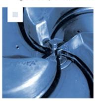
bends their path into circular orbits. Each revolution, the ions receive three 140,000-volt electric jolts, which add energy and widen the orbit. The ions are then passed to the larger K1200 cyclotron, where they are stripped of more electrons and accelerated to speeds up to 93,000 miles per second. having travelled almost three miles in 0.00006 seconds.
