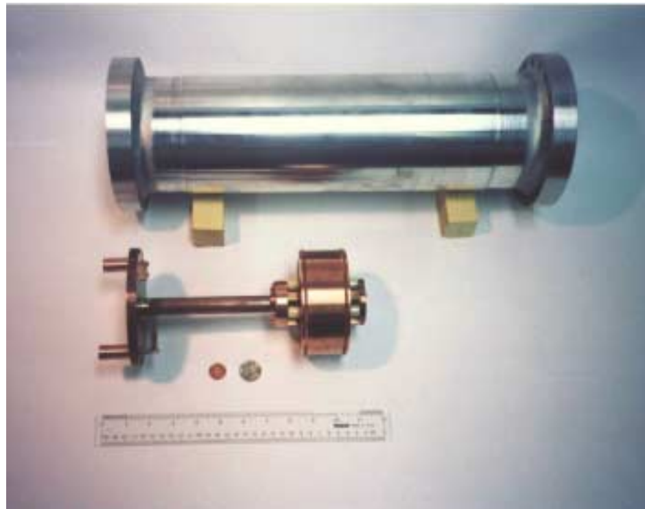
Figure 78. Components of the hybrid rf cavity. Here the magnetron is assembled. The magnetron, inner conductor, and shorting plate (all made of copper) are about to be inserted into the aluminum outer conductor.
