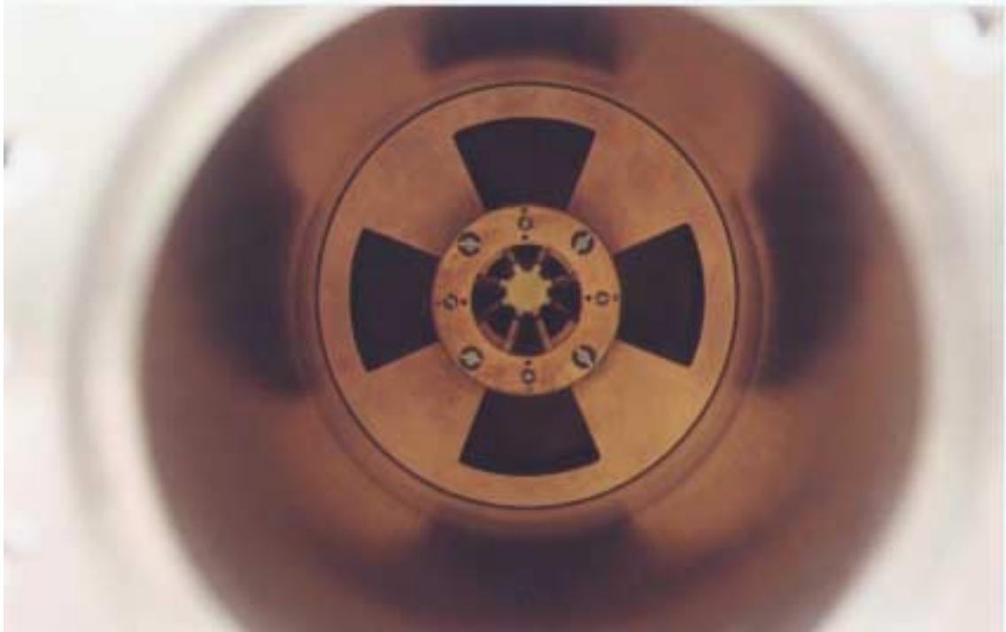
Figure 79. A view of the fully assembled rf cavity looking into the extraction end. The 8 tapered magnetron vanes of the acceleration section can be seen inside the ID of the exit mounting ring.
