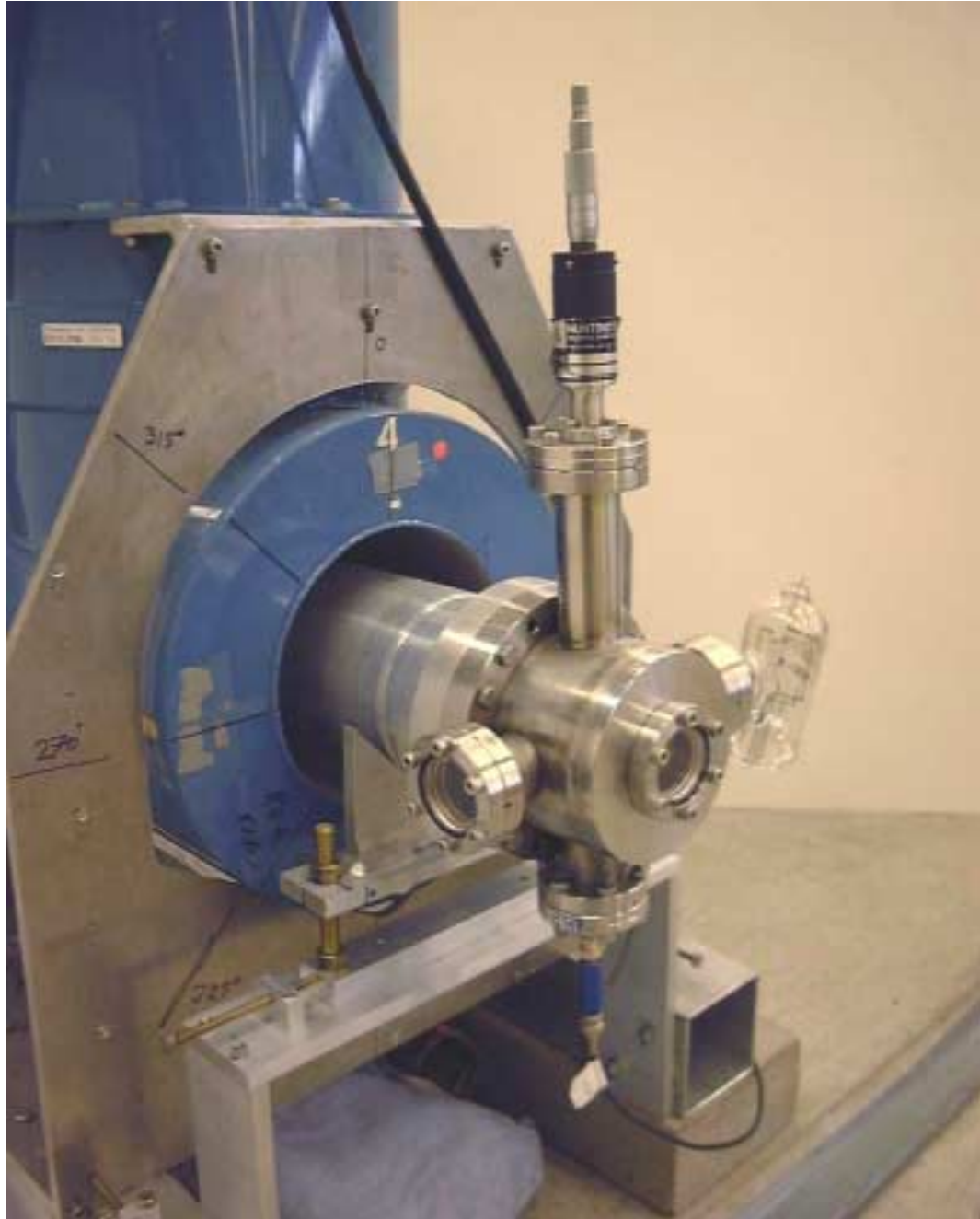
Figure 71. The extraction end of the 50 keV ICRA. The rf accelerating cavity (aluminum tube) is mounted in the bore of the superconducting magnet (blue). The V-block below the cavity can be adjusted in order to align the rf cavity with the magnetic axis. The extraction port covers the extreme downstream end of the system and contains the extraction Faraday cup and viewports for observing the beam. The mechanical feedthrough on top of the extraction port is used to move the radial probe, in the radial direction (see Figure 73).
