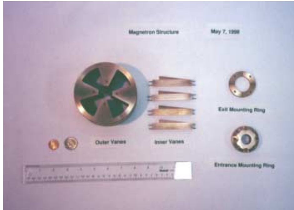
Figure 77. Components of the magnetron section before assembly.
