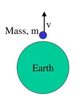
The velocity to completely escape the gravity of a planet is:  $KE(leaving) = PE(far \ away)$   $\frac{1}{2}mv^{2} = \frac{GmM_{planet}}{planet}$
