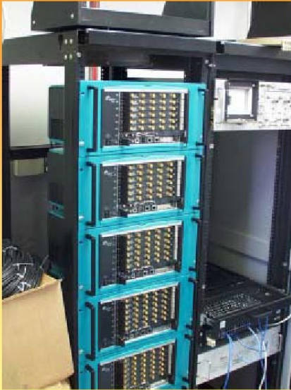
320 channels read out electronics
